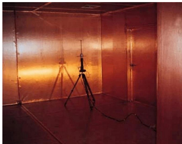
Fig 8: Measuring the premises shielding efficiency
