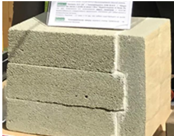
Fig 10: Radio-absorbing construction material based on foamed ceramics Ceramopen™.
